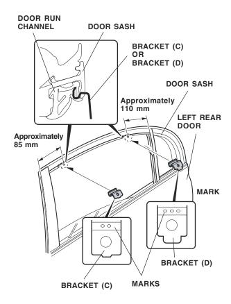
Install a bracket (C) and a bracket (D) on the door sash at the measurements shown. Verify the shape and the identification mark stamped on each bracket. Be sure to use the correct bracket at the proper location. Position the left rear door visor on the door sash.
