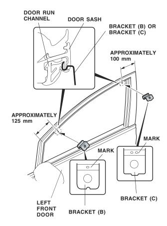
18. Install a bracket (B) and a bracket (C) on the door sash at the measurements shown. Verify the shape and the identification mark stamped on each bracket. Be sure to use the correct bracket at the proper location.
