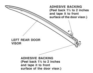
12. Align the hole in the visor with the mark you made on the masking tape, and install the clips.
