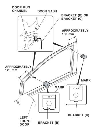
18. Install one bracket (B) and one bracket (C) on the door sash at the measurements shown. Verify the shape and the identification mark stamped on each bracket. Be sure to use the correct bracket at the proper location.
