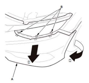
4. With the help of an assistant, while pulling the front bumper (A) away from the side spacer, release the bumper from the hooks (B) on the upper beam.
