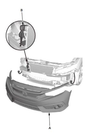
NOTE: When installing the front bumper (A), take care not to bend the front bumper side induction plate (B).
