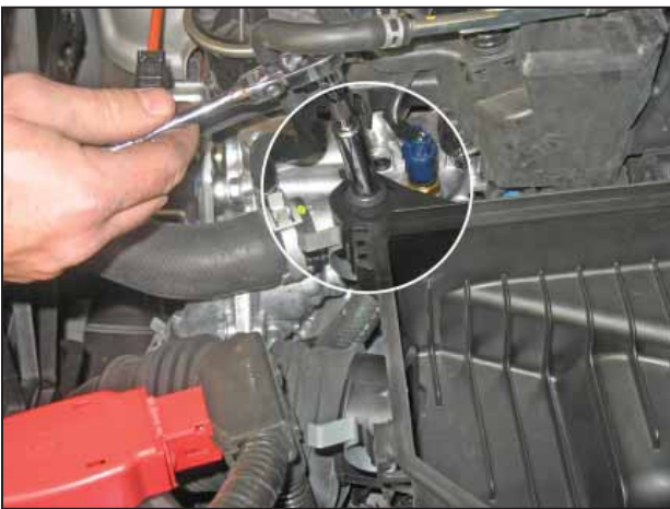
i. Remove the front bolt securing the stock airbox.
