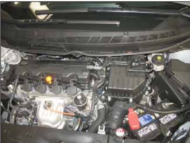
Stock airbox system installed
