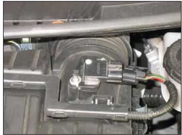
b. Disconnect the mass airflow sensor harness from the mass airflow sensor.
