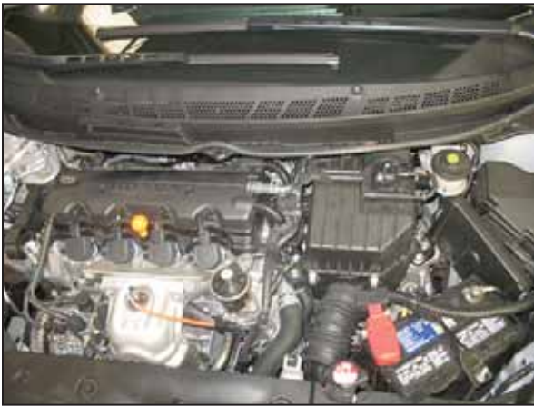
a. Stock airbox system installed.
