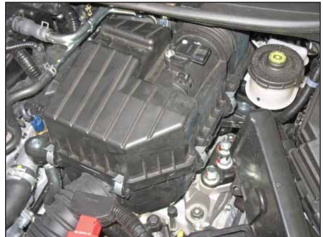
d. Unclip the metal clips securing the airbox lid to the lower airbox.
