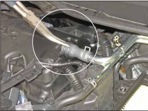
g. Disconnect the PCV hose from the valve cover.
