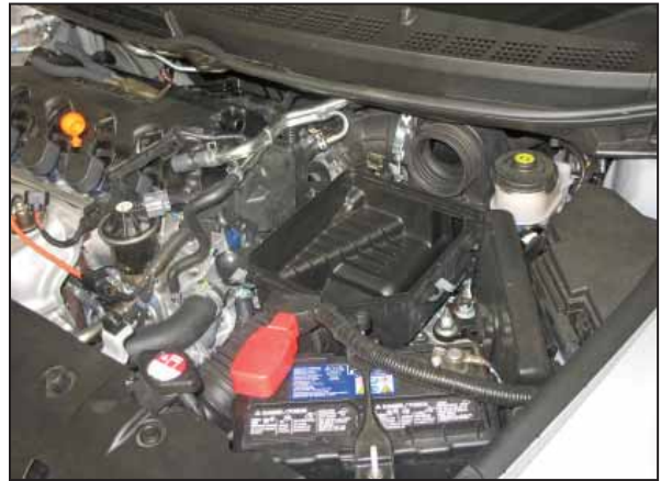
h. Remove the stock panel air filter.
