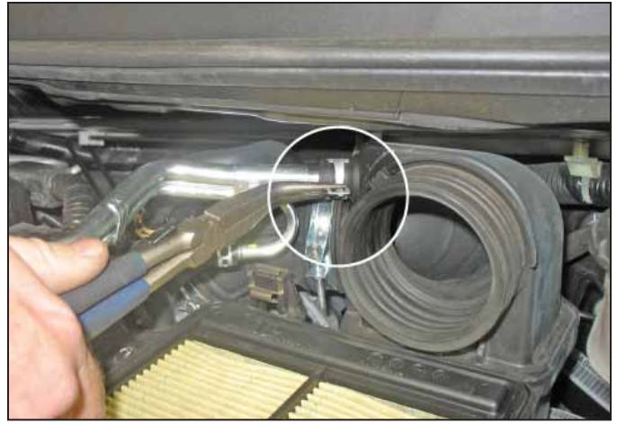
f. Disconnect the PCV hard line from the rubber inlet.
