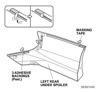
12. Using one alcohol swab, thoroughly clean the rear bumper where the left rear under spoiler will attach.
