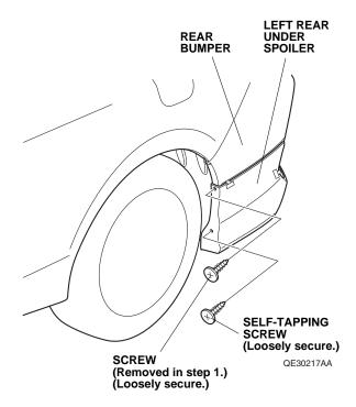
15. While applying light pressure against the left rear under spoiler, carefully remove the adhesive backings.
