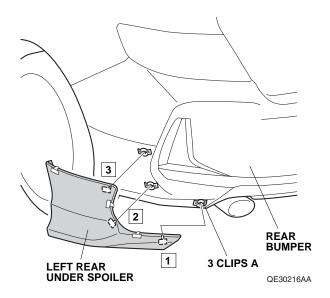
14. Loosely secure the left rear under spoiler to the rear bumper with one self-tapping screw and the screw removed in step 1.
