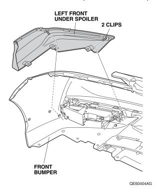
Secure the left front under spoiler with two clips.
