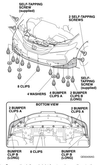
Secure the left and right front under spoilers to the front bumper with four bumper clips A, two bumper clips B (long), four washers, and two self-tapping screws.
