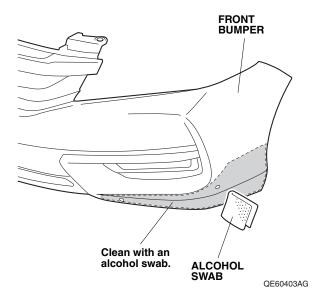
9. Install the left front under spoiler to the front bumper.
