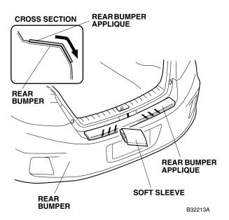
14. Using a shop towel, wipe up the 3M protective tape application solution. Allow the rear bumper applique to dry thoroughly.
