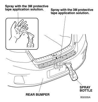
5. Remove the adhesive backing from the side of the rear bumper applique with the 3M mark.
