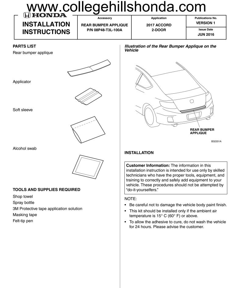
1. Open the trunk lid. Use the alcohol swab to thoroughly clean the area where the rear bumper applique will attach.
