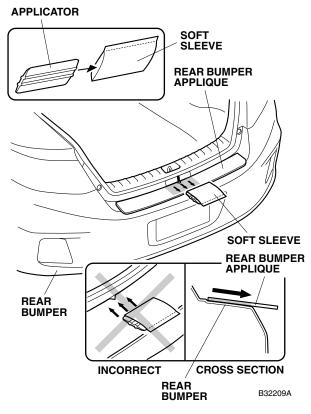
9. Starting from the front and working rearward, use the soft sleeve to smooth out the center of the upper section on the rear bumper applique. Move the soft sleeve in one direction only. If you see an air bubble, stop and gently peel up that section to work out the bubble. Work slowly and keep pressure against the rear bumper applique.
