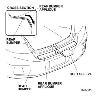
13. Repeat step 10 to smooth the left and right sides of the lower section on the rear bumper applique.
