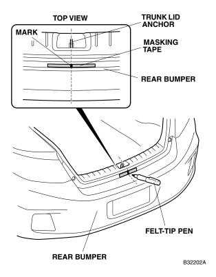
Align the rear bumper applique with the rear bumper and check the rear bumper applique position.
