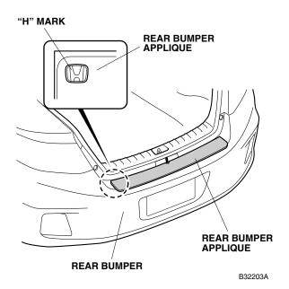
4. Using a spray bottle with the 3M protective tape application solution, spray the area where the rear bumper applique will attach. Spray some solution on your hands.
