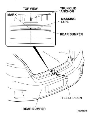
Align the rear bumper applique with the rear bumper and check the rear bumper applique position. Remove the rear bumper applique.
