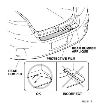
12. Repeat step 9 at the center of the lower section of the rear bumper applique.
