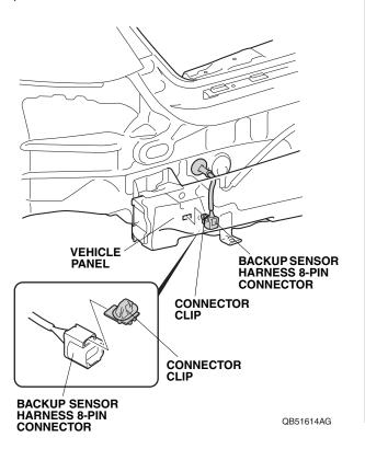
41. With the help of an assistant, bring the rear bumper next to the vehicle, plug the subharness 8-pin connector into the backup sensor harness 8-pin connector, and reinstall the rear bumper.
