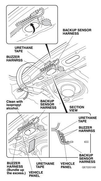
25. Bundle up the excess buzzer harness, and secure the buzzer harness and backup sensor harness to the vehicle panel with one urethane tape as shown.
