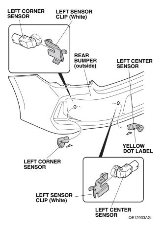
12. Using the sensor clips, install the right corner sensor into the 24 mm hole and the right center sensor into the 26 mm hole in the rear bumper. Note the direction and the pin location for each sensor.
