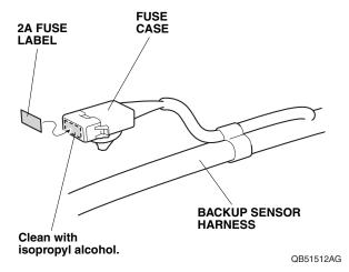
Secure the backup sensor harness to the vehicle harness with one wire tie.
