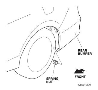
13. Install the left rear splash guard to the rear bumper with two washer-screws and the screw removed in step 7. Install them in this order ☐ → ② → ③. Make sure there is no gap between the left rear splash guard and the vehicle body. If there is a gap, loosen the two washer-screws and one screw, hold the splash guard against the body, and tighten the two washer-screws and one screw.
