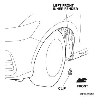
4. Install the left front splash guard to the left front inner fender with two washer-screws and the clip removed in step 3. Install them in this order 1→2→3. Make sure there is no gap between the left front splash guard and the vehicle body. If there is a gap, loosen the two washer-screws, hold the splash guard against the body, and tighten the two washer-screws.
