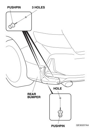
While wearing eye protection, drill the four pierced marks to 8 mm. First drill with a 3 mm drill bit, next with a 6 mm drill bit, and finish with an 8 mm drill bit.
