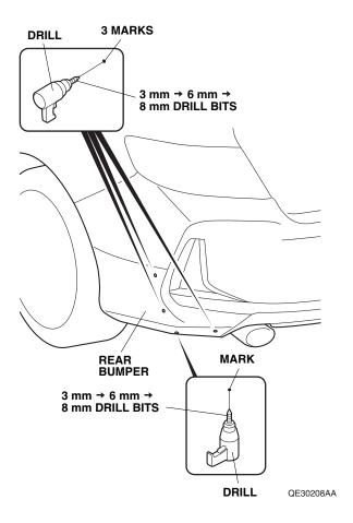
5. Enlarge the three upper holes to 12 mm using a 12 mm drill bit. Remove any burrs.
