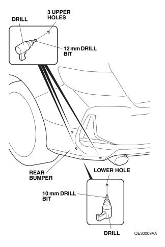
6. Enlarge the lower hole to 10 mm using a 10 mm drill bit. Remove any burrs.
