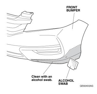
9. Install the left front under spoiler to the front bumper.
