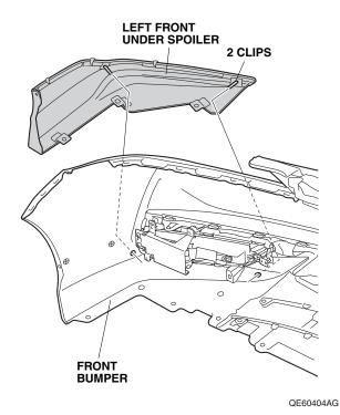
10. Secure the left front under spoiler with two clips. NOTE: Do not push the clip too tightly, or it may deform the left front under spoiler. Readjust the clips, if necessary.
