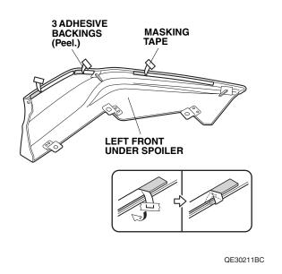
8. Using one alcohol swab, thoroughly clean the front bumper where the left front under spoiler will attach.
