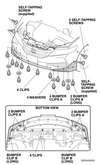
14. Secure the left and right front under spoilers to the front bumper with four bumper clips A, two bumper clips B (long), four washers, and two self-tapping screws.
