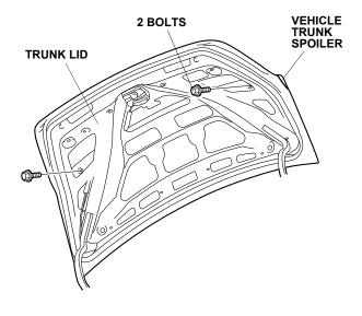
4. Close the trunk lid. Release the vehicle trunk spoiler (eleven clips).
