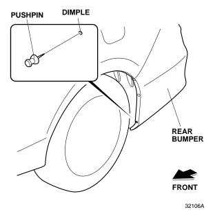
9. Gently pull away the rear bumper in the area shown. Using a felt-tip pen, mark the left rear inner fender at the measurement shown.
