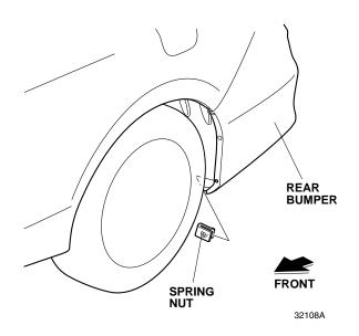
13. Install the left rear splash guard to the rear bumper with two new washer-screws and the washer-screw removed in step 7. Install them in this order
