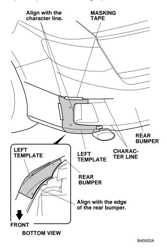
3. Using a pushpin, pierce the rear bumper through the four holes in left template. Remove the left template.
