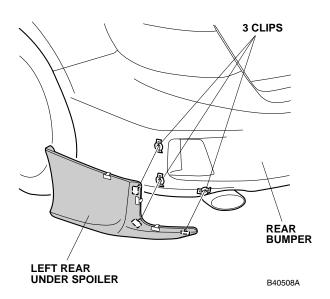
While applying light pressure against the left rear under spoiler, carefully remove the adhesive backings.
