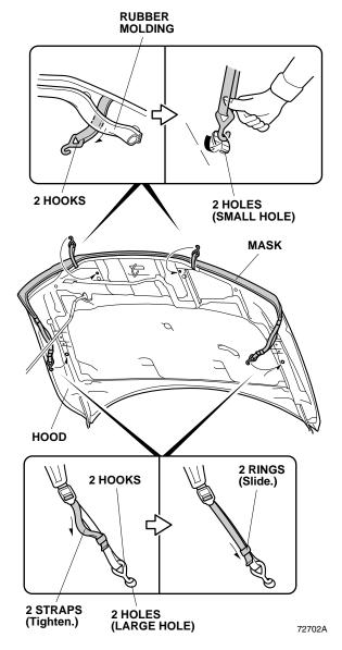
2. Route the two center hooks under the rubber molding, and attach them to each hole (small hole) on the hood.
