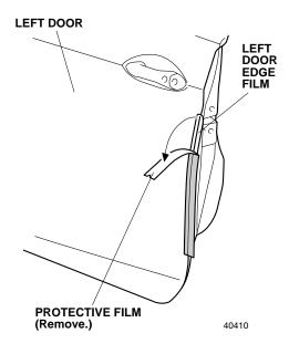
8. Starting from the center and working outward, use your finger to fold the left door edge film inside the left door. Move your finger in one direction only. Do not damage the door seam sealant.
