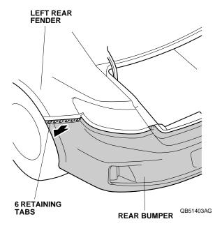
Release the three retaining tabs on each side of the bumper.
