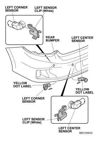
12. Using the sensor clips, install the right corner sensor and right center sensor into the 24 mm hole and 26 mm hole in the rear bumper. Note the direction and the pin location for each sensor.
