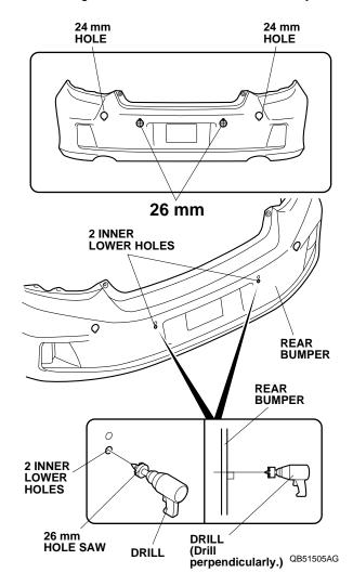
11. Using the sensor clips, install the left corner sensor and left center sensor into the 24 mm hole and 26 mm hole in the rear bumper. Note the direction and the pin location for each sensor.
