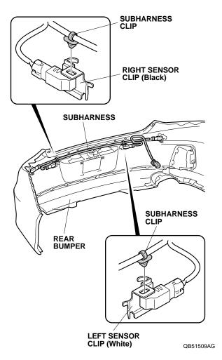
15. Using isopropyl alcohol on a shop towel, thoroughly clean the rear bumper where the aluminum tapes will attach.
