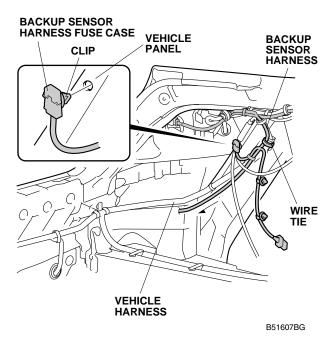
30. Secure the backup sensor harness to the vehicle harness with one wire tie.
