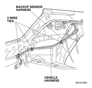
If equipped with vehicle harness, install the wire tie with holder to the backup sensor harness 8-pin connector, and secure it to the vehicle harness. Go to step 41.
