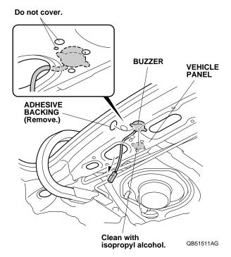
18. Remove the adhesive backing from the buzzer and attach it to the vehicle panel.
