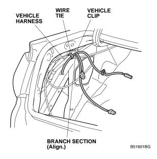
21. Secure the clip on the backup sensor harness to the vehicle panel.
