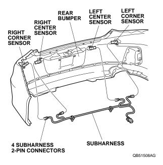
14. Secure the two subharness clips to the left sensor clip and right sensor clip as shown.
