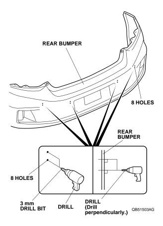
Using a 24 mm hole saw, enlarge the outboard (left and right corner sensor) bumper holes by drilling the upper 3 mm holes. Remove any burrs.
