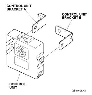
32. Secure the control unit to the vehicle panel with the flange bolt at the location shown.
