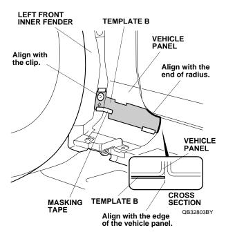
10. Using a felt-tip pen, mark the vehicle panel in the area shown. Remove template B. Be careful not to damage the template. It is also used to mark the right side of the vehicle.
