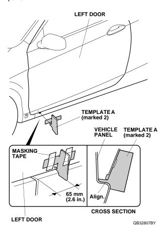
16. Using a felt-tip pen, mark the vehicle panel at the measurement shown.
