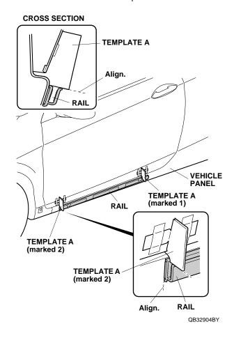
21. Make sure that the rail is aligned with each template, then carefully remove each adhesive backing.
