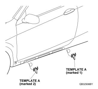
23. Using the palm of your hand, firmly press the rail against the vehicle panel for 30 seconds. Remove the mark you made using isopropyl alcohol on a shop towel.
