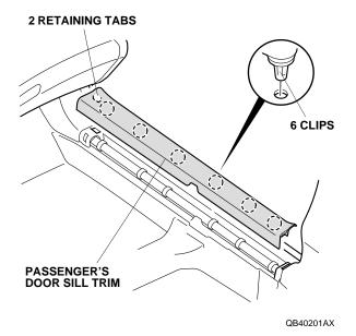
Pull away the door opening seal, and remove the passenger's kick panel (two clips).
