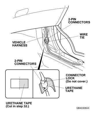
50. Secure the 2-pin connectors to the vehicle harness with one wire tie.
