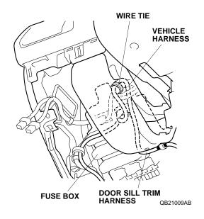
39. Release the driver's console side cover (one hook and one clip).
