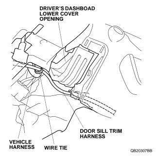
45. On the passenger's side of the vehicle, route the door sill trim harness and secure it to the vehicle harness with two wire ties.
