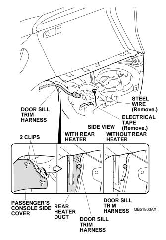
42. Route the door sill trim harness, and remove the electrical tape and steel wire.
