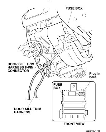
28. Remove and discard the dummy connector from the other accessory harness. Plug the door sill trim 8-pin connector into the other accessory harness 8-pin connector.
