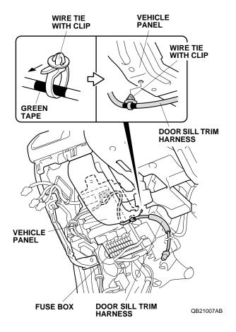
36. Using diagonal cutters, cut the clip portion off of one wire tie.
