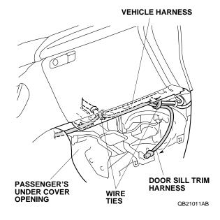
46. Route the door sill trim harness and secure it to the vehicle panel and vehicle harness with two wire ties.
