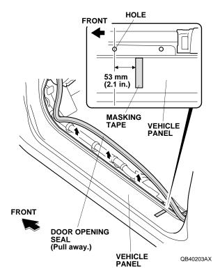
12. Attach a piece of masking tape to the vehicle panel in the location shown.
