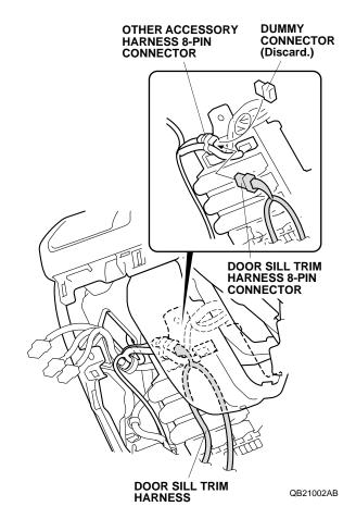
29. Route the door sill trim harness as shown, and secure the door sill trim harness to the vehicle harness with two wire ties.
