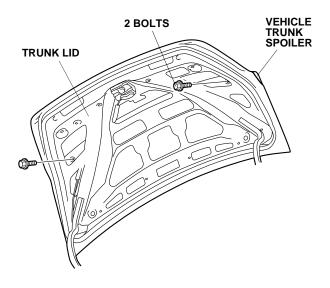
Close the trunk lid. Release the vehicle trunk spoiler (eleven clips).
