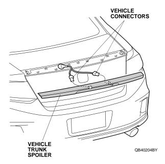
8. Remove the high-mount brake light from the vehicle trunk spoiler (three self-tapping screws). Set the vehicle trunk spoiler aside, it will not be reused.
