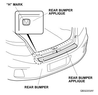
4. Using a spray bottle with the 3M protective tape application solution, spray the area where the rear bumper applique will attach. Spray some solution on your hands.
