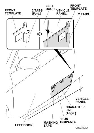
Insert the folded tabs of the front template into the opening between the left door and the vehicle panel.
