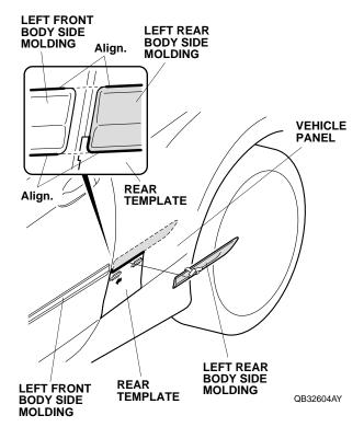
14. Check that the edges of the front and rear moldings are aligned. Readjust the moldings if necessary.
