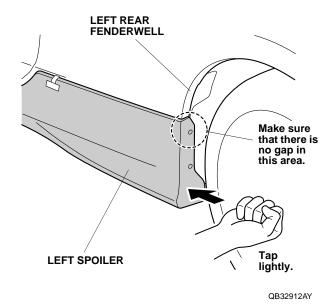
29. Install two flare nuts to the rear fenderwell. Install the flare nuts in the correct position and orientation. Loosely install two self-tapping screws.
