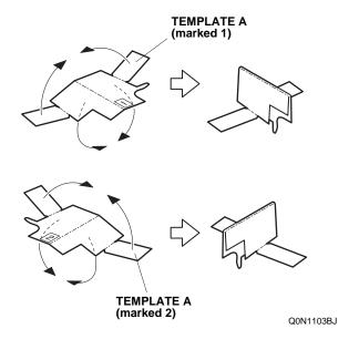
15. Place template A (marked 2) into position at the location shown. Align template A with the vehicle panel; lightly push down on the template, and attach it to the left door with masking tape. Make sure there is no gap between the template and the vehicle panel.
