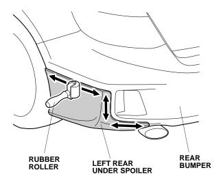
12. Secure the left rear under spoiler with one bumper clip and one clip removed in step 1.
