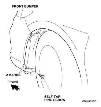
8. Install one spring nut over each hole in the front bumper in the direction shown.
