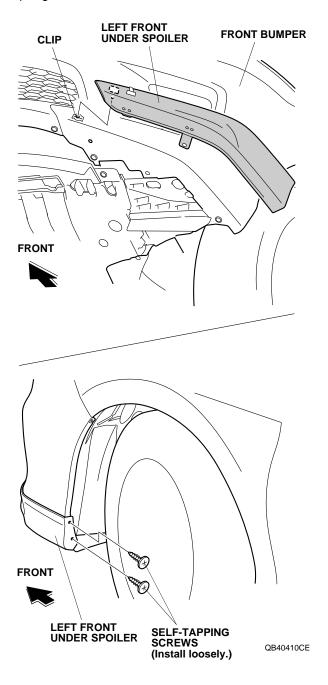
Secure the front portion of the left front under spoiler to the front bumper with one washer and one bumper clip supplied.
