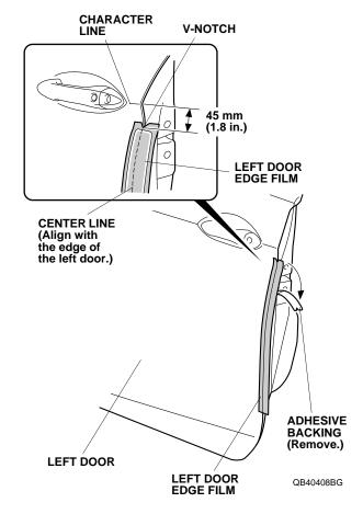
5. Align the center line on the left door edge film with the edge of the left door. While applying light pressure, carefully remove the adhesive backing.
