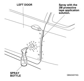
4. Open the left door. Peel back about 50 mm (2.0 in.) of adhesive backing from the left door edge film. Align the V-notch on the left door edge film 45 mm (1.8 in.) below the character line.
