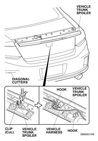
6. Release the vehicle harness from the vehicle trunk spoiler.
