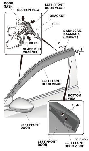
10. Using a soft towel, press and hold the left front door visor against the door sash and left front door for 30 seconds.
