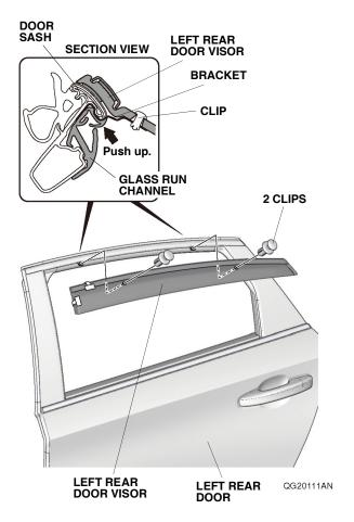
17. Using the two clips, secure the left rear door visor to the brackets as shown. Make sure to push up on the brackets while installing the two clips.
