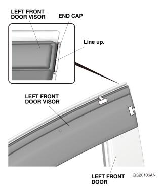
9. While applying light pressure against the left front door visor, carefully remove the taped adhesive backings in the order shown.
