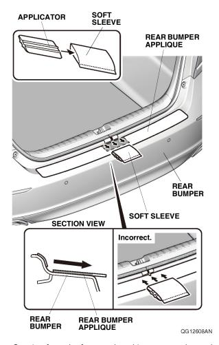
8. Starting from the front and working rearward, use the soft sleeve to smooth out the center of the upper section on the rear bumper applique. Move the soft sleeve in one direction only. If you see an air bubble, stop and gently peel up that section to work out the bubble. Work slowly, and keep pressure against the rear bumper applique.
