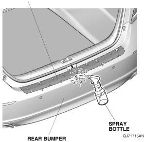
4. Remove the adhesive backing from the side of the rear bumper applique.
