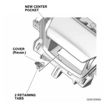
69. Install the wireless charger unit in the new center pocket with two retaining tabs and four self-tapping screws.
