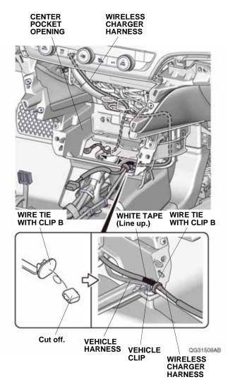
56. Line up the white tape on the wireless charger harness with the vehicle clip, and secure the wireless charger harness to the vehicle harness with one wire tie with clip B as shown.
