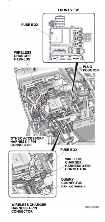
46. Route the wireless charger harness. Secure the wireless charger harness 12-pin connector to the fuse box.
