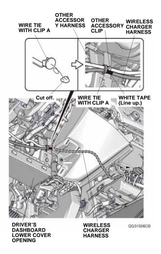
51. Line up the white tape on the wireless charger harness with the other accessory clip, and secure the wireless charger harness to the other accessory harness with one wire tie with clip A as shown.
