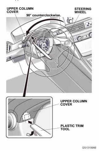
10. Turn the steering wheel 180° clockwise. Using a plastic trim tool, release the upper column cover.
