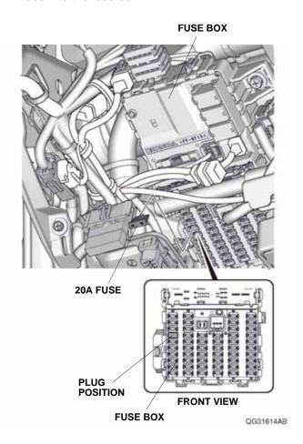
73. Using isopropyl alcohol on a shop towel, thoroughly clean the fuse label where the fuse label B will attach. Attach the fuse label B (20A OPTION FUSE) to the fuse label on the driver's kick panel as shown.
