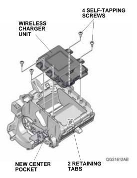
70. Install the right side panel and left side panel. Plug the wireless charger harness 7-pin connector to the wireless charger unit.
