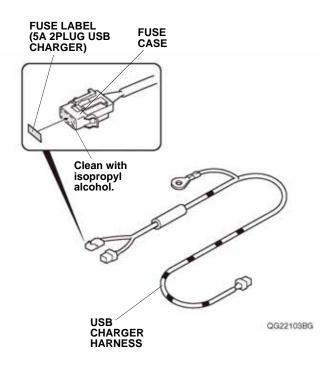
27. Route the USB charger harness as shown, and plug the USB charger harness 4-pin connector into the fuse box. If another accessory harness 4-pin connector is plugged into the fuse box, remove the dummy connector from that accessory harness 4-pin connector, and plug the USB charger harness 4-pin connector into that connector.
