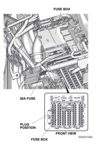
66. Using isopropyl alcohol on a shop towel, thoroughly clean the fuse label where the fuse label will attach. Attach the fuse label (20A OPTION FUSE) to the fuse label on the driver's kick panel as shown.
