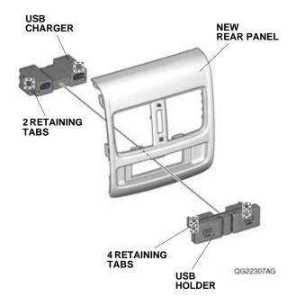
60. Install the new rear panel to the rear console panel with the six retaining tabs.
