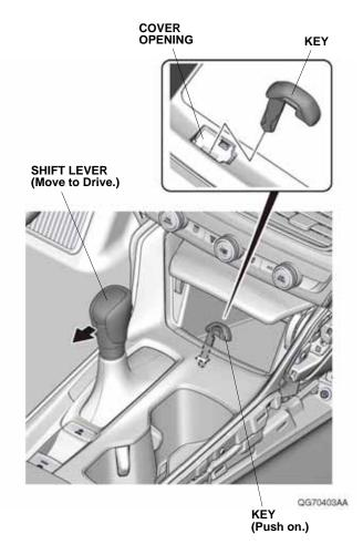
19. Remove the key and install the cover. Close the lid.
