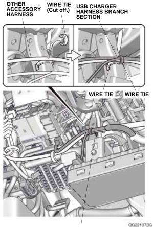
USB CHARGER HARNESS If the vehicle is equipped with another accessory harness, go to step 32; otherwise, continue with step 31.
