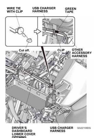
33. Line up the green tape on the USB charger harness with the other accessory harness clip, and secure the USB charger harness to the other accessory harness with one wire tie with clip as shown. 34. Route the USB charger harness along the vehicle frame. Remove the vehicle ground bolt, and secure the USB charger harness ground terminal to the vehicle ground terminals with vehicle ground bolt just removed.
