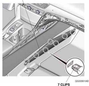
4. Remove the driver's dashboard lower cover and unplug the vehicle connectors.
