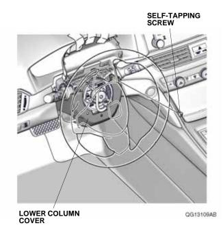
11. Turn the steering wheel 180° counterclockwise, and remove the other self-tapping screw from the lower column cover.
