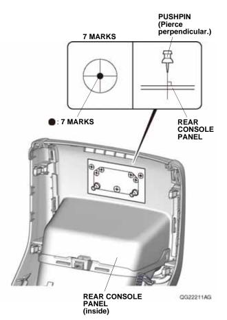
47. Using a utility knife, mark the rear console panel along the printed line in the template. Remove the template.
