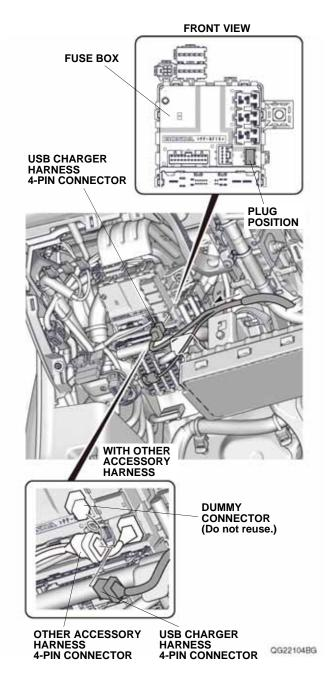
28. Secure the fuse case on the USB charger harness to the fuse box. If another accessory harness is secured on the fuse box, remove the other accessory harness from the fuse box. Secure the fuse case on the USB charger harness to the fuse box, then secure the other accessory harness to the fuse case on the USB charger harness as shown.
