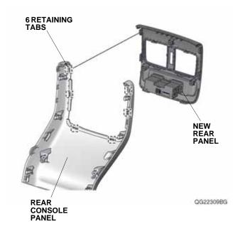
61. Install the duct to the rear console panel with the six retaining tabs and five screws removed in step 57.
