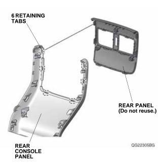
59. Install the USB holder and USB charger to the new rear panel with the six retaining tabs.
