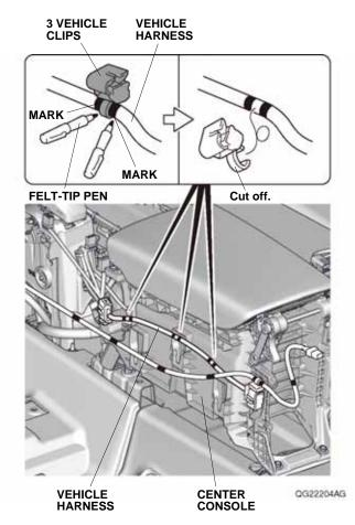
38. Cut off the three vehicle clips from the vehicle harness.NOTE: Be careful not to damage the vehicle
