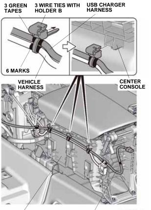
CENTER CONSOLE USB CHARGER HARNESS 40. Secure the USB charger harness to the vehicle connectors with one wire tie with holder A at the green tape on the USB charger harness as shown.
