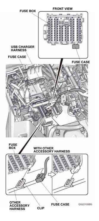
If the vehicle is equipped with another accessory harness, go to step 30; otherwise, continue with step 29.
