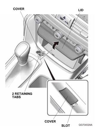
18. Insert the key into the cover opening. Push on the key and move the shift lever to Drive.
