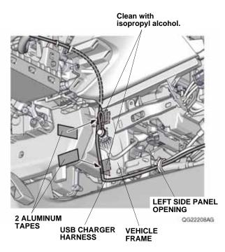
43. Secure the USB charger harness to the vehicle frame with two pieces of aluminum tape.
