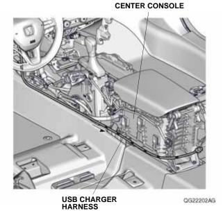
36. Secure the USB charger harness to the vehicle connector with one wire tie with holder A at the green tape on the USB charger harness as shown.
