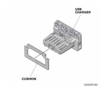
Install the USB charger to the rear console panel with two screws as shown.
