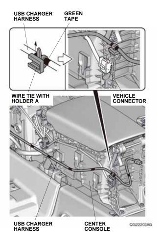
37. Using a felt-tip pen, mark the vehicle harness at each clip as shown.
