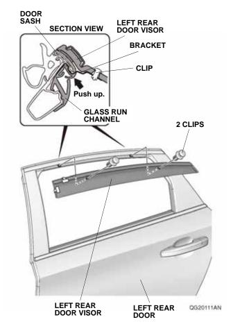
17. Using the two clips, secure the left rear door visor to the brackets as shown. Make sure to push up on the brackets while installing the two clips.
