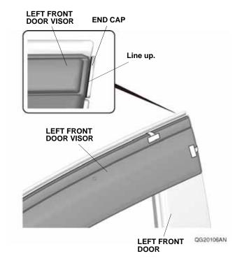
9. While applying light pressure against the left front door visor, carefully remove the taped adhesive backings in the order shown.
