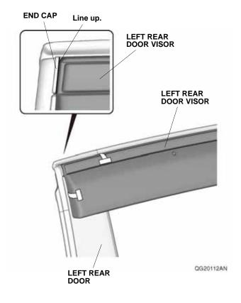
While applying light pressure against the left rear door visor, carefully remove the taped adhesive backings in the order shown.
