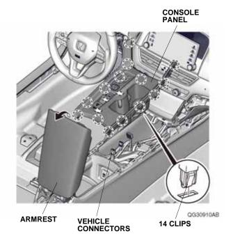
28. Remove the center pocket, and unplug the vehicle connectors.
