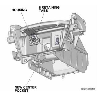
67. Install the accessory power socket in the housing with two retaining tabs.
