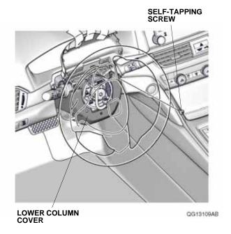
13. Turn the steering wheel 180° counterclockwise, and remove the other self-tapping screw from the lower column cover.
