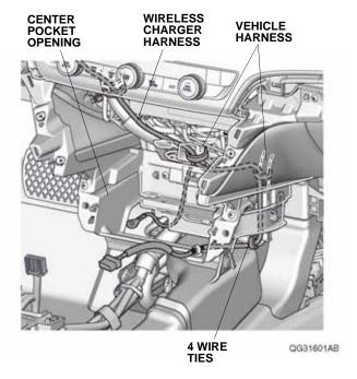
58. Remove the vehicle ground bolt, and secure the wireless charger harness ground terminal to the vehicle ground terminals with vehicle ground bolt. Do not put the ground terminal calkings on top of one another.
