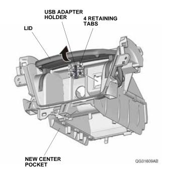
66. Install the housing in the new center pocket with eight retaining tabs.
