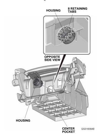
If the vehicle is equipped with the center pocket light, continue with step 63; if not go to step 65.
