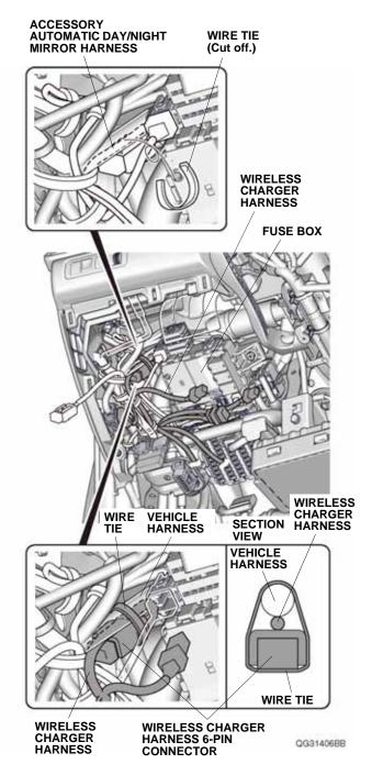
37. Secure the wireless charger harness 6-pin connector to the vehicle harness with one wire tie as shown.
