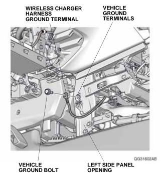
59. Secure the wireless charger harness to the vehicle harness with one wire tie.
