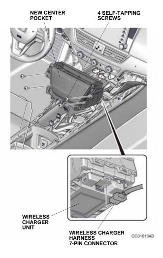
71. Install the new center pocket with four self-tapping screws removed in step 28.
