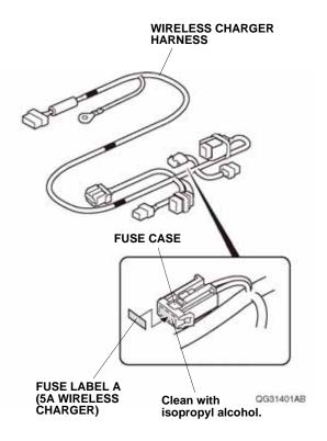
32. Line up the branch section of the wireless charger harness with the vehicle clip. Secure the wireless charger harness to the vehicle harness with two wire ties.
