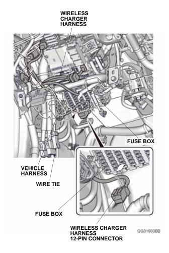
47. Secure the wireless charger harness to the vehicle harness with one wire tie.
