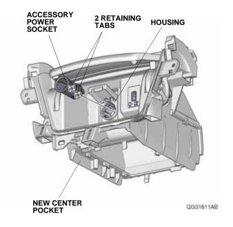
68. Install the cover removed in step 19 in the new center pocket with two retaining tabs.
