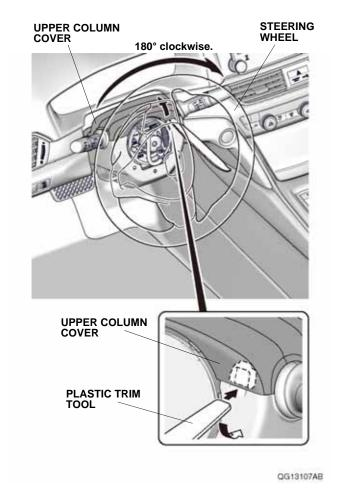
11. Release the upper column cover and secure it to the dashboard with masking tape.
