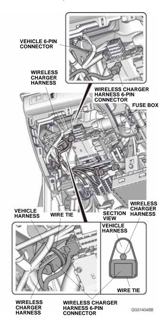
35. Secure the wireless charger harness 6-pin connector to the vehicle harness with one wire tie as shown. Go to step 44.
