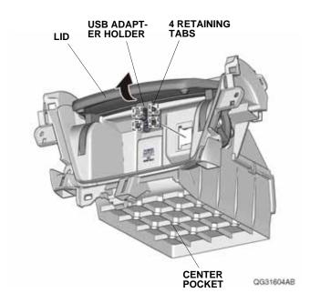
61. Open the housing cover, and remove the accessory power socket.
