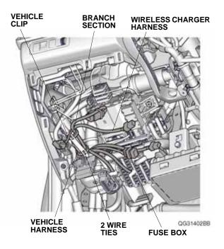
33. Secure the fuse case to the vehicle connectors.
