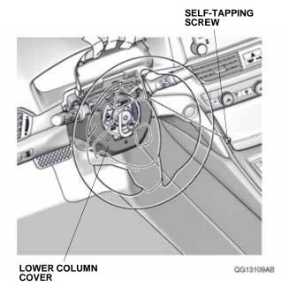
11. Turn the steering wheel 180° counterclockwise, and remove the other self-tapping screw from the lower column cover.
