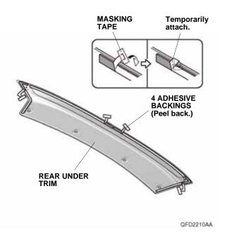
Line up the rear under trim with the rear bumper as shown. Loosely install the rear under trim to the rear bumper with four clips, two washers, and two selftapping screws.
