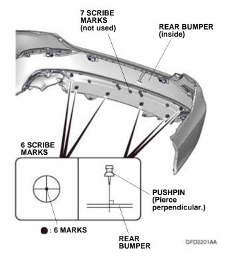
4. While wearing eye protection, drill the six pierced marks to 8 mm. First, drill with a 3 mm drill bit, then follow with a 6 mm drill bit, and finish with an 8 mm drill bit.
