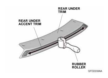
11. Using an alcohol wipe, thoroughly clean the rear bumper where the rear under trim will attach. NOTE: Any remaining oil or dirt on the rear bumper surface will affect the adhesive tape effectiveness, which could cause gaps or lifting of the rear under trim.
