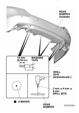
5. While wearing eye protection, enlarge the four drilled holes on the rear bumper to 10 mm with a 10 mm drill bit
