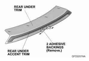
Using a rubber roller, apply firm pressure against the rear under accent trim and roll from one end to the other.
