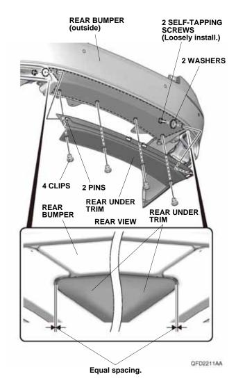
14. While applying light pressure against the rear under trim, carefully remove the taped adhesive backings.
