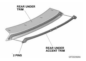
While applying light pressure against the rear under accent trim, carefully remove the taped adhesive backings.
