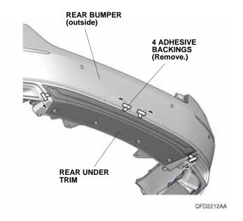
Using a rubber roller, apply firm pressure against the rear under trim and roll from one end to the other. NOTE: Apply firm pressure, especially at the ends.
