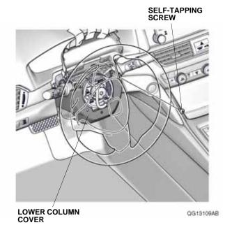
24. Turn the steering wheel 180° counterclockwise, and remove the other self-tapping screw from the lower column cover.
