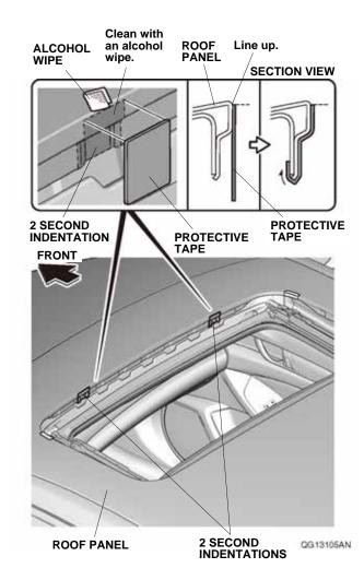
6. Remove the adhesive backings from two pieces of protective tape, and attach one to the roof panel at each second indentation.
