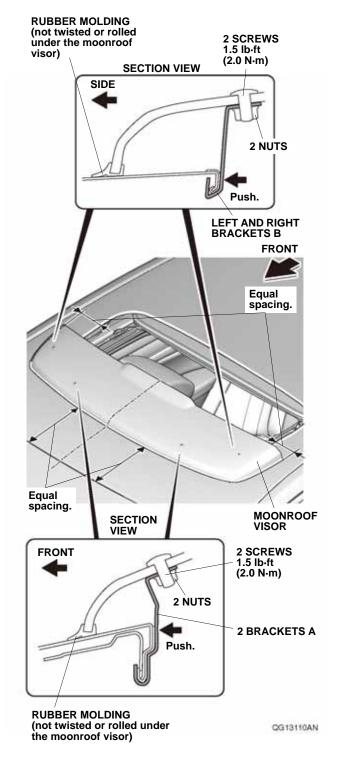
12. Tighten the two screws and two nuts on the front of the vehicle first, then tighten the two screws and two nuts on each side. Tighten while applying pressure so there is no gap between the roof panel and the brackets A and B. Torque the screws to 1.5 lb·ft (2.0 N·m).
