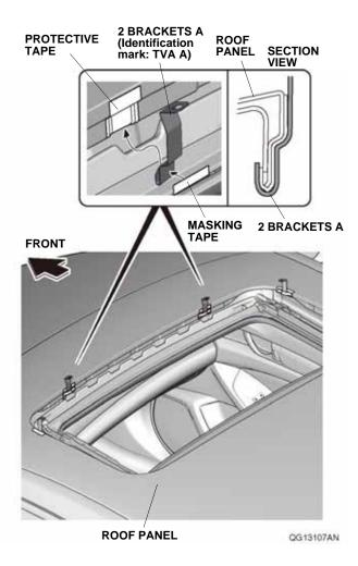
9. Set the moonroof visor on the roof in front of the moonroof opening, and adjust its position so the holes in the moonroof visor are lined up with the holes in brackets A. Loosely install the moonroof visor to brackets A with two screws and two nuts. Remove the strips of masking tape from brackets A.
