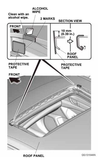
4. Remove the adhesive backings from two pieces of protective tape, and attach one to the roof panel at each of the two marks you made. Wrap 10 mm (0.39 in.) of the protective tape around the lip of the moonroof opening.
