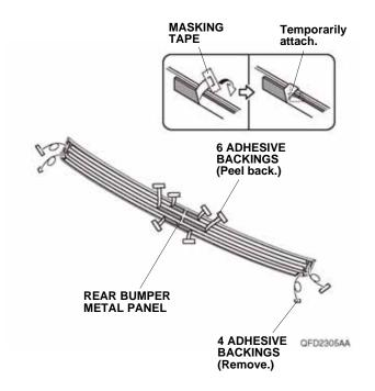
6. Attach the rear bumper metal panel to the rear bumper by lining it up with the masking tape as shown.
