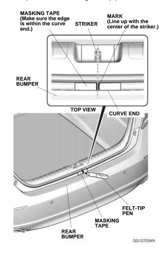
2. Line up the mark on the sticker with the mark on the masking tape. Then, attach masking tape at both ends as shown.
