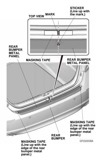
3. Remove the rear bumper metal panel from the rear bumper.
