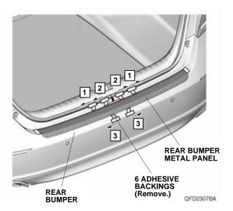
8. Using a rubber roller, apply firm pressure against the rear bumper metal panel and roll from one end to the other.
