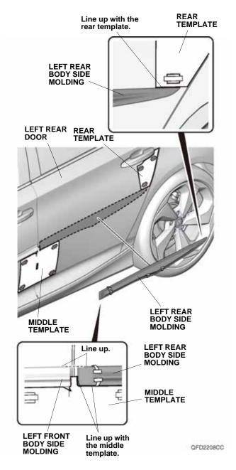
12. Make sure the edges of the left front body side molding and left rear body side molding are lined up.
