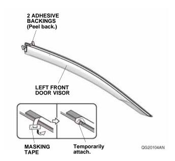
6. Adjust the two brackets so the holes line up with the two holes in the left front door visor.
