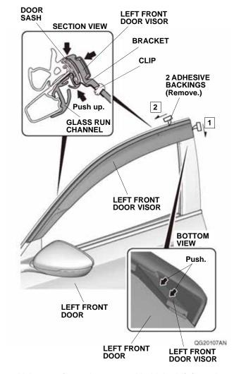
Using a soft towel, press and hold the left front door visor against the door sash and left front door for 30 seconds.
