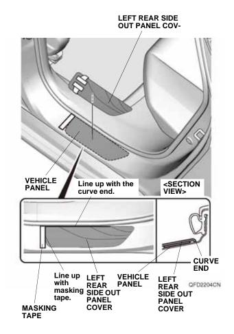
12. While applying light pressure against the left rear side out panel cover, carefully remove the taped adhesive backings.
