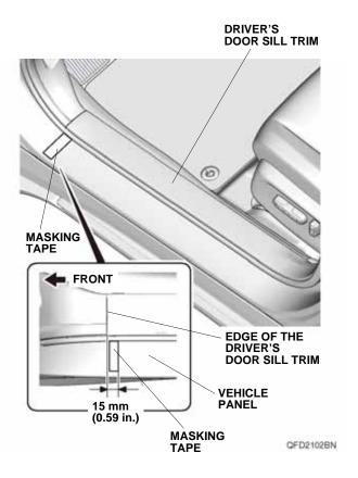
2. Using an alcohol wipe, thoroughly clean the vehicle panel where the left front side out panel cover will attach.
