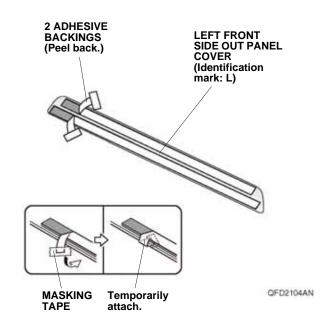
4. Line up the left front side out panel cover with the masking tape and curve end as shown. Attach the left front side out panel cover to the vehicle panel.
