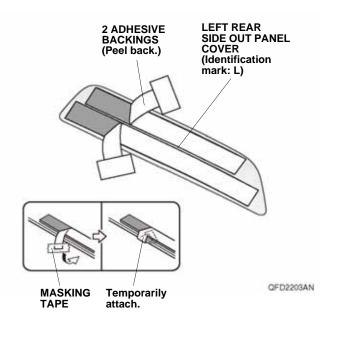
11. Line up the left rear side out panel cover with the masking tape and curve end as shown. Attach the left rear side out panel cover to the vehicle panel.
