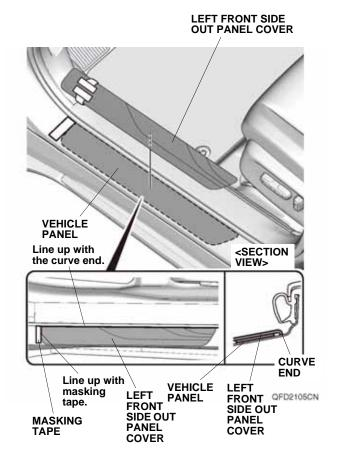
5. While applying light pressure against the left front side out panel cover, carefully remove the taped adhesive backings.
