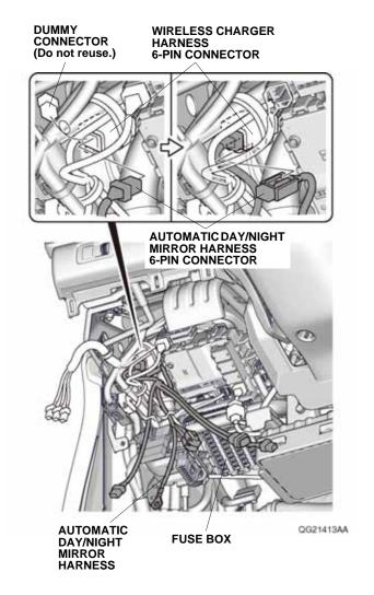
18. Secure the automatic day/night mirror harness 6-pin connector to the wireless charger harness 6-pin connector. Go to step 26.
