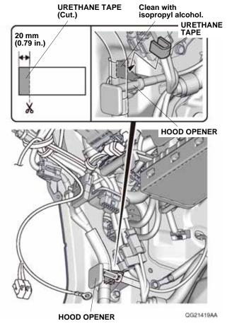
30. Using scissors, cut the urethane tape as shown and attach the 20 mm piece of urethane tape to the hood opener as shown.
