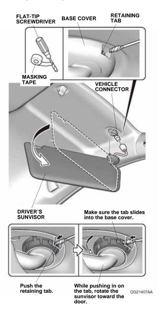
7. Remove the driver's sunvisor holder by rotating it 45° counterclockwise.
