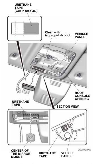
43. Attach the urethane tape cut in step 36 to the vehicle panel as shown.
