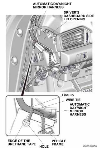
38. Secure the automatic day/night mirror harness to the vehicle harness with one wire tie.
