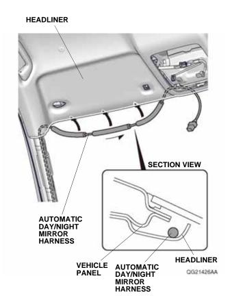
41. Secure the automatic day/night mirror harness to the vehicle harness with two wire ties as shown.
