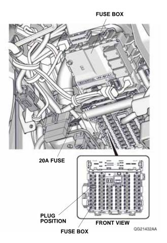
48. Using isopropyl alcohol on a shop towel, thoroughly clean the fuse label where the fuse label will attach. Attach the fuse label (20A OPTION FUSE) to the fuse label on the driver's kick panel as shown.
