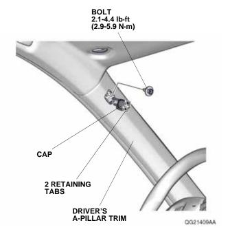
9. Pull away the door opening seal and remove the driver's A-pillar trim.
