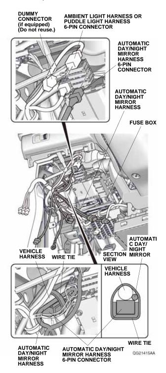
22. Secure the automatic day/night mirror harness 6-pin connector to the vehicle harness with one wire tie as shown. Go to step 26.
