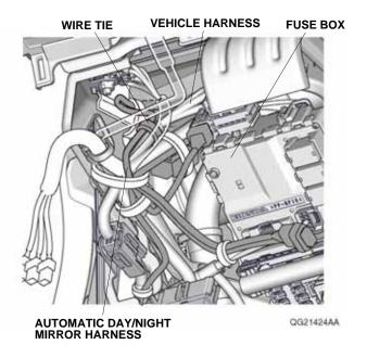
39. Route the automatic day/night mirror harness behind the vehicle harness. Line up the green tape on the automatic day/night mirror harness with the vehicle clip, and secure the automatic day/night mirror harness to the vehicle harness with one wire tie as shown.
