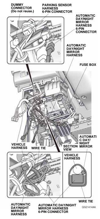
20. Secure the automatic day/night mirror harness 6-pin connector to the vehicle harness with one wire tie as shown. Go to step 26.
