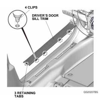
13. Pull away the door opening seal and remove the driver's kick panel.
