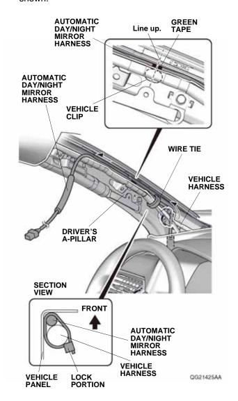
40. Route the automatic day/night mirror harness along the driver's A-pillar. Gently pull back the headliner, and tuck the automatic day/night mirror harness behind the headliner.
