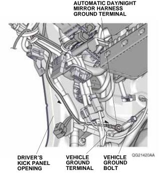
32. Remove the vehicle ground bolt. Secure the automatic day/night mirror harness ground terminal and the vehicle ground terminal with the bolt just removed.
