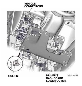
11. Pull away the door opening seal and remove the driver's dashboard side lid.
