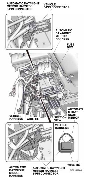
16. Secure the automatic day/night mirror harness 6-pin connector to the vehicle harness with one wire tie as shown. Go to step 26.
