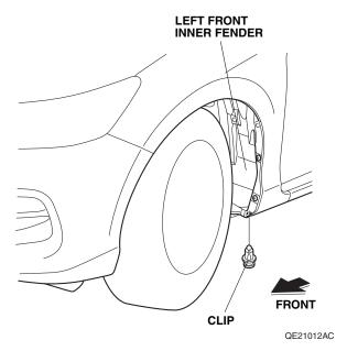
4. Install the left front splash guard to the left front inner fender in this order 1→2→3 using the two washer-screws and the clip removed in step 3. If necessary, trim the under sealant. Make sure there is no gap between the left front splash guard and the vehicle body. If there is a gap, loosen the three screws, hold the splash guard against the body, and tighten the three screws.
