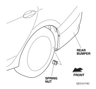
13. Install the left rear splash guard to the rear bumper in this order 1→2→3 using the two washer-screws and one screw removed in step 7. Make sure there is no gap between the left rear splash guard and the vehicle body. If there is a gap, loosen the three screws, hold the splash guard against the body, and tighten the three screws.
