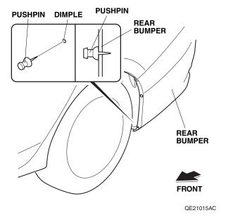
9. Pull away the rear bumper. Cut the left rear inner fender in the area shown.
