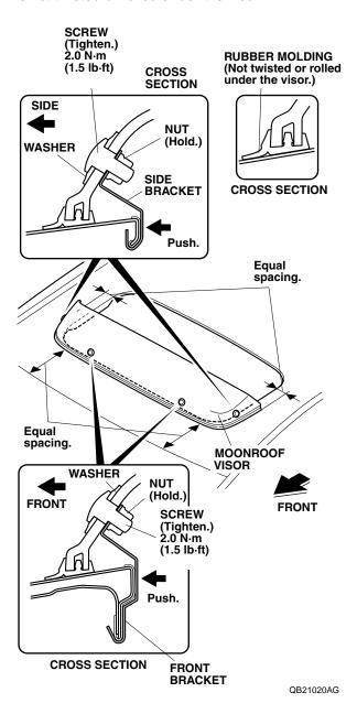
17. Tighten the two screws on the side of the opening first, then tighten the two screws on the front. Apply pressure so that there is no gap between the brackets and the roof panel. Torque the screws to 2.0 N·m (1.5 lb·ft).
