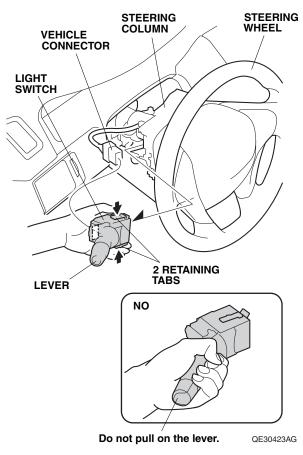
9. Push down on the two retaining tabs, slide the light switch out, and remove it from the steering column. Do not pull on the lever.
