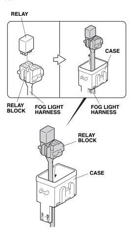
36. Route the fog light harness through the case, and install the relay block in the case.
