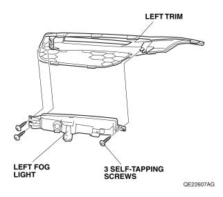
21. Install the left trim on the front bumper with nine retaining tabs and one clip.
