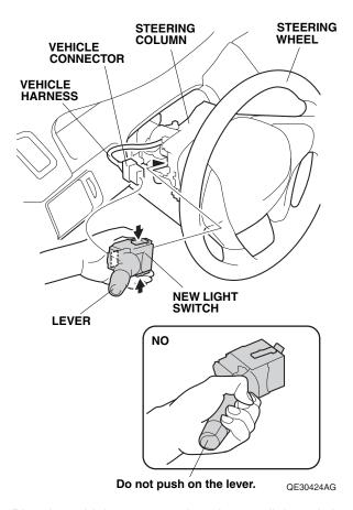
Plug the vehicle connector into the new light switch. Make sure the vehicle harness is not being stretched.
