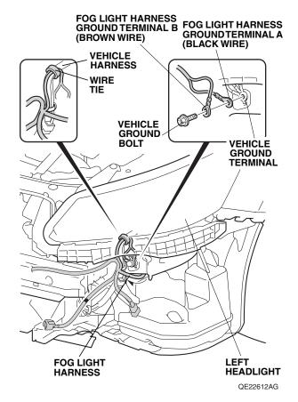
43. Secure the fog light harness to the vehicle harness with one wire tie.
