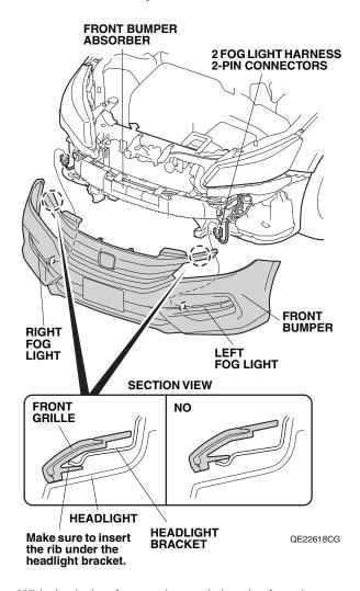
52. With the help of an assistant, bring the front bumper close to the vehicle. Plug the two fog light harness 2-pin connectors into the left fog light and right fog light, then reinstall the front bumper.
