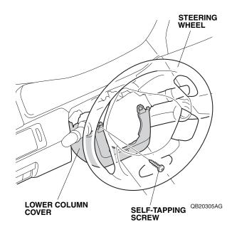
6. Turn the steering wheel 180° clockwise, and remove the other self-tapping screw from the lower column cover.
