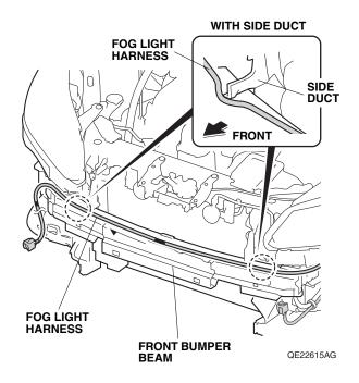
48. Align the green tape on the fog light harness with the vehicle clip, and secure the fog light harness to the vehicle harness with one wire tie.
