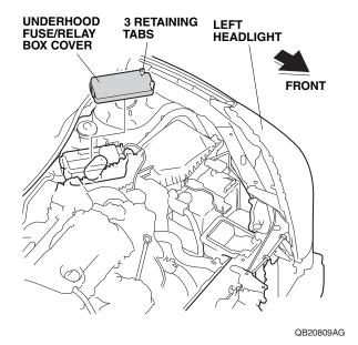
54. Plug the 10 A fuse into the under-hood fuse/relay box.
