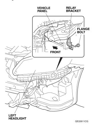
41. Install the case on the relay bracket.
