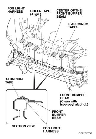
50. Align the green tape on the fog light harness with the center of the front bumper beam, and secure the fog light harness to the front bumper beam with six aluminum tapes.
