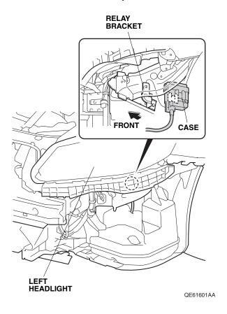
42. Route the fog light harness as shown. Remove the vehicle ground bolt, and secure the fog light harness ground terminals A and B to the vehicle ground terminal. Install the vehicle ground bolt.
