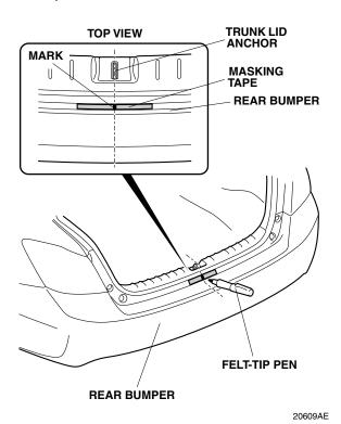
Align the rear bumper applique with the rear bumper and check the rear bumper applique position.
