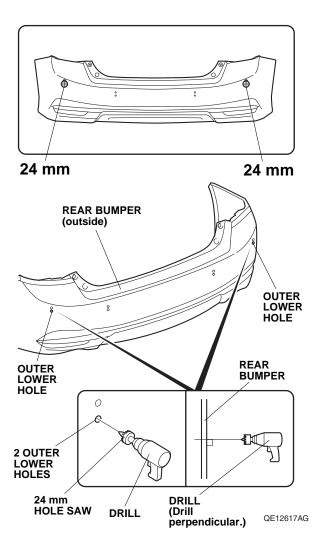
Using a 26 mm hole saw, enlarge the inboard (center sensor) bumper holes by drilling the lower 3 mm holes. Remove any burrs.
