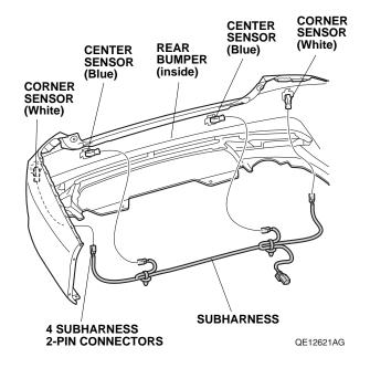
Secure the two subharness clips to the two center sensor clips as shown.
