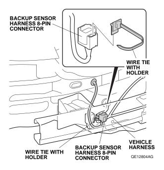
51. Install the connector clip to the backup sensor harness 8-pin connector, and secure it to the vehicle panel.
