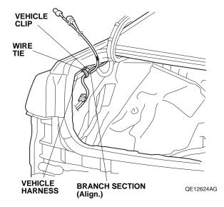
35. Align the green tape on the backup sensor harness with the vehicle clip, and secure the backup sensor harness to the vehicle harness with one wire tie as shown.
