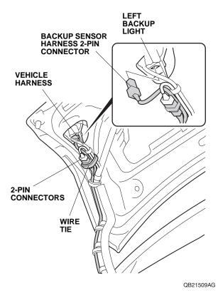
40. Secure the 2-pin connectors to the vehicle harness with one wire tie.
