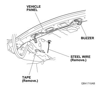
28. Using isopropyl alcohol on a shop towel, thoroughly clean the vehicle panel where the buzzer will attach.
