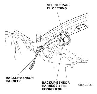
34. Secure the backup sensor harness to the vehicle harness with one wire tie.
