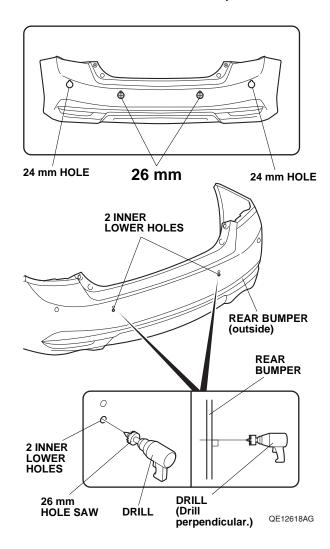
17. Using the two center sensor clips, install the two center sensors (Blue) into the 26 mm holes in the rear bumper. Note the direction and the pin location for each sensor.
