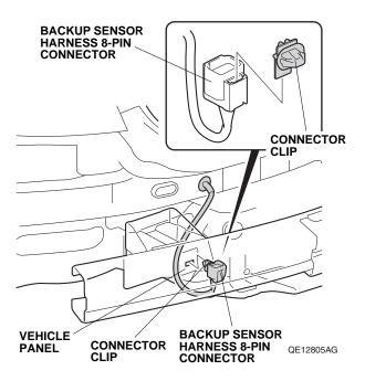
52. With the help of an assistant, bring the rear bumper next to the rear of the vehicle, plug the subharness8-pin connector into the backup sensor harness8-pin connector, and install the rear bumper.
