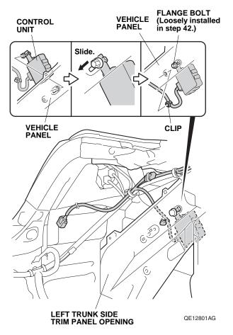
45. Secure the clip on the backup sensor harness to the vehicle panel.
