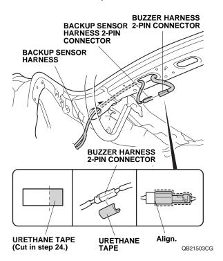
32. Wrap the remaining piece of urethane tape (cut in step 24) around the buzzer harness 2-pin connector.
