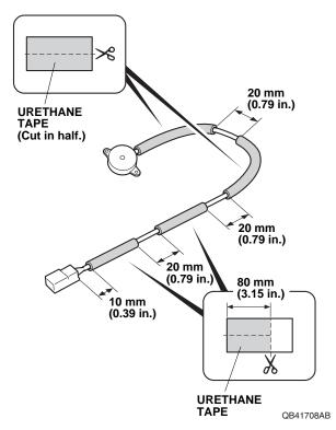
24. Using scissors, cut one urethane tape into three pieces. Wrap two of the pieces of urethane tape around the buzzer harness as shown.
