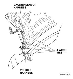
38. Unplug the vehicle 2-pin connector (Green) from the left backup light, and plug it into the backup sensor harness 2-pin connector.
