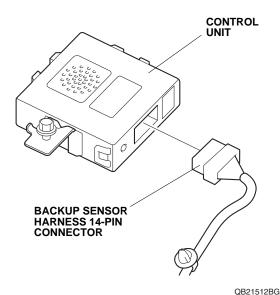
44. Secure the control unit to the vehicle panel with the flange bolt loosely installed in step 42 as shown.
