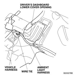
19. On the passenger's side of the vehicle, route and secure the ambient light harness to the vehicle harness with two wire ties.
