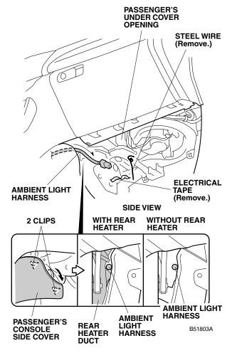
16. Route the ambient light harness as shown, then remove the electrical tape and steel wire.
