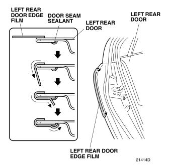
Using a shop towel, wipe the excess 3M protective tape application solution from the left rear door edge film. Allow the left rear door edge film to dry thoroughly.
