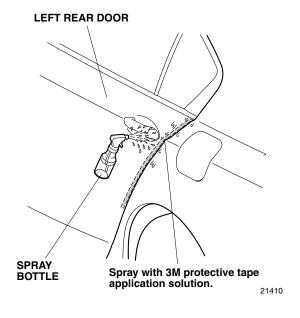
13. Open the left rear door. Peel back about 50 mm (2.0 in.) of adhesive backing from the left rear door edge film. Align the V-notch on the left rear door edge film with the left rear door as shown.
