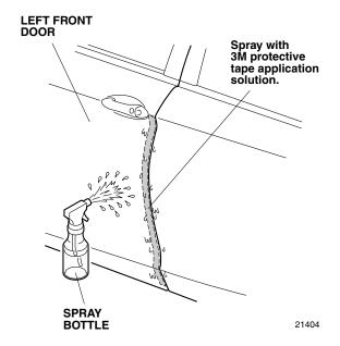
Open the left front door. Peel back about 50 mm (2.0 in.) of adhesive backing from the left front door edge film. Align the V-notch on the left front door edge film with the character line on the left front door.
