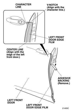
Align the center line on the left front door edge film with the edge of the left front door. While applying light pressure, carefully remove the adhesive backing. 8. Insert the applicator into the soft sleeve. Starting from the center and working outward, use the soft sleeve to smooth out the left front door edge film. Move the soft sleeve in one direction only.
