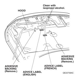
25. Remove the adhesive backings from the advice labels, and attach the two advice labels to the hood as shown.
