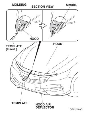
23. Open the hood. Tighten the two 5 x 9.5 mm truss screws and the two 6 x 12 mm screws loosely installed in steps 10 and 11.
